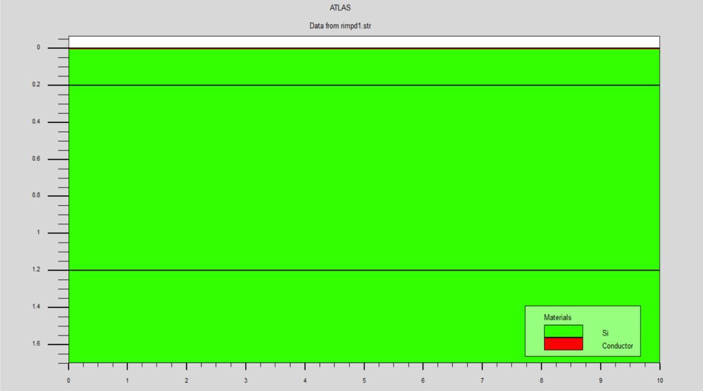
Fig . 3.1 Structure of PIN photodetector
