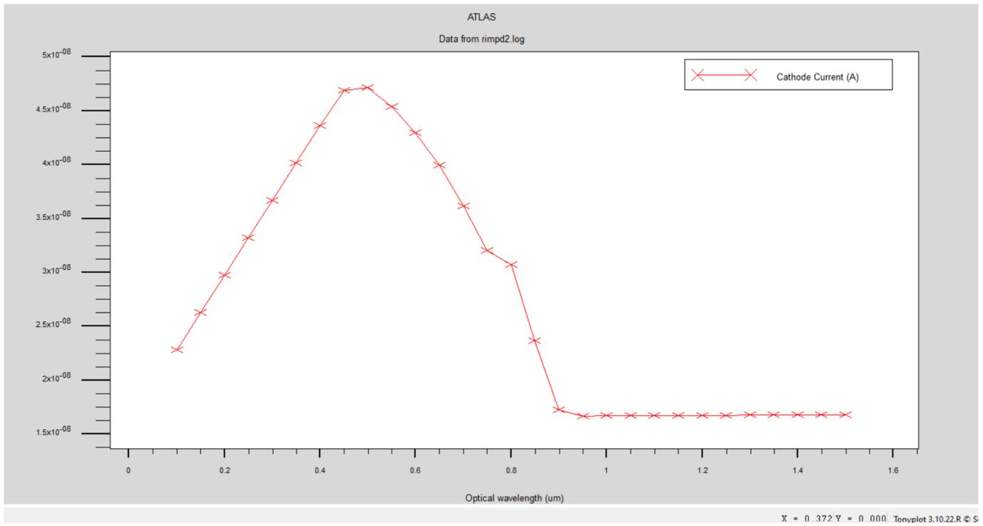
Fig . 5.7 Plot Between Optical Wavelength Vs Cathode current for GaAs/InGaAs/Si
