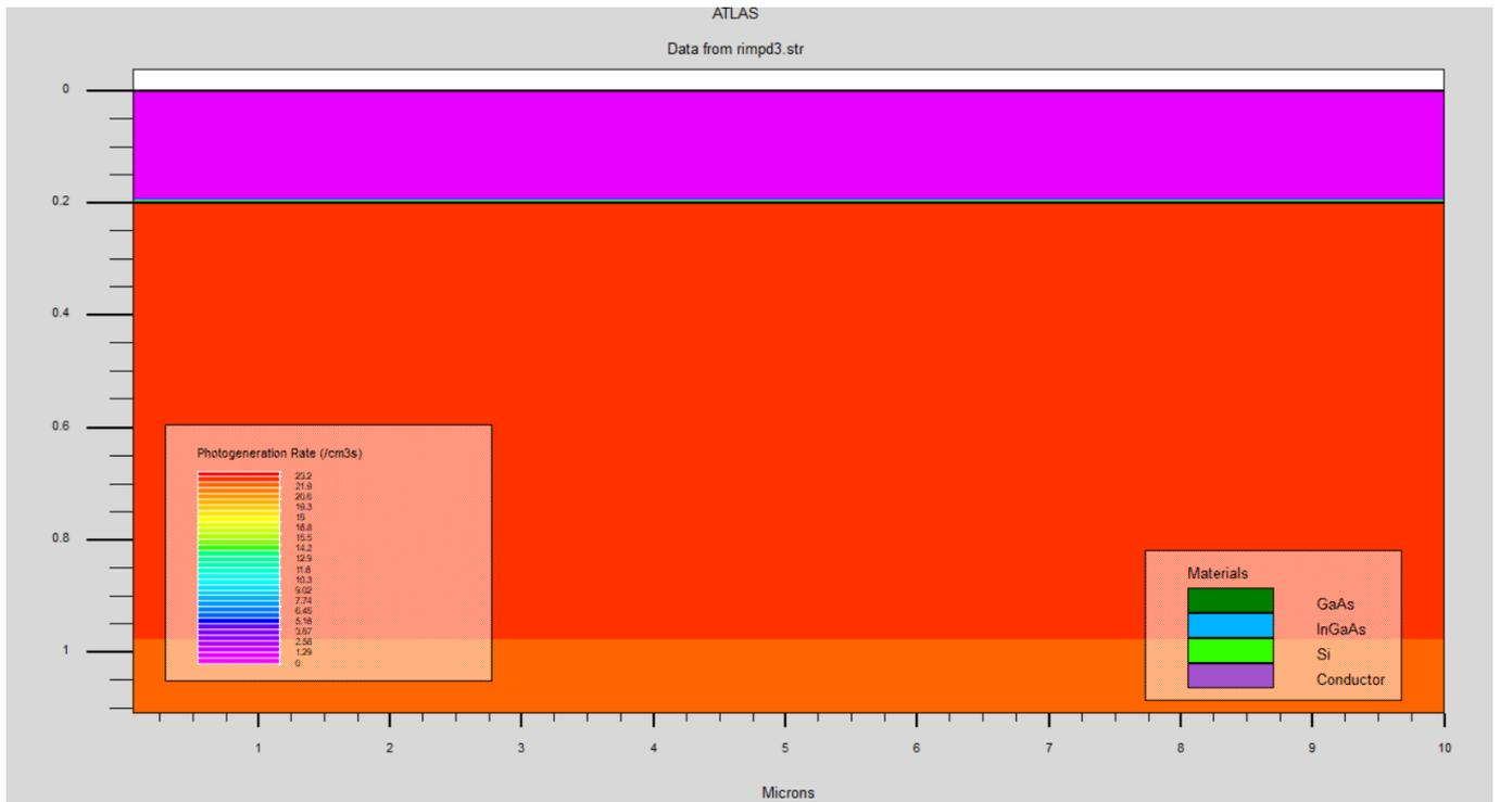
Fig 5.12: Photogeneration rate of GaAs/InGaAs/Si after increasing the intrinsic layer
