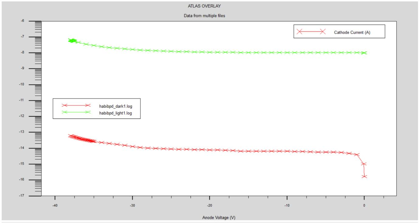
Fig . 5.11 Plot Between Anode Voltage Vs Cathode Current for Si after increasing the intrinsic layer
