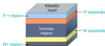
Fig : 2.2 Structure of PIN
