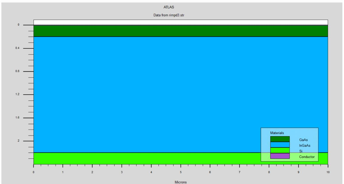
Fig 5.12: Structure of GaAs/InGaAs/Si after increasing the intrinsic layer
