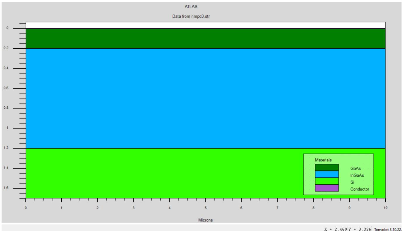
Fig . 5.5 Structure of GaAs/InGaAs/Si
