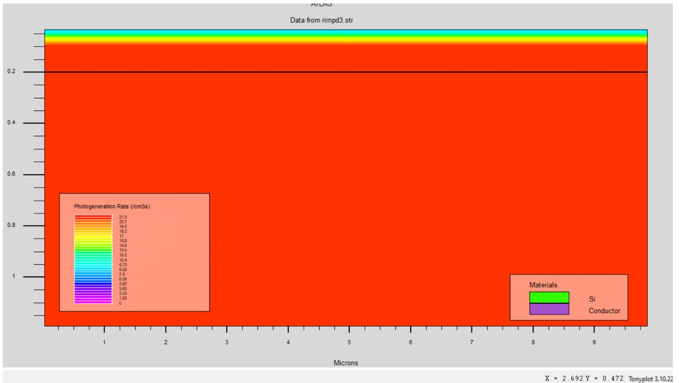
Fig . 5.2 photogeneration rate for Si
