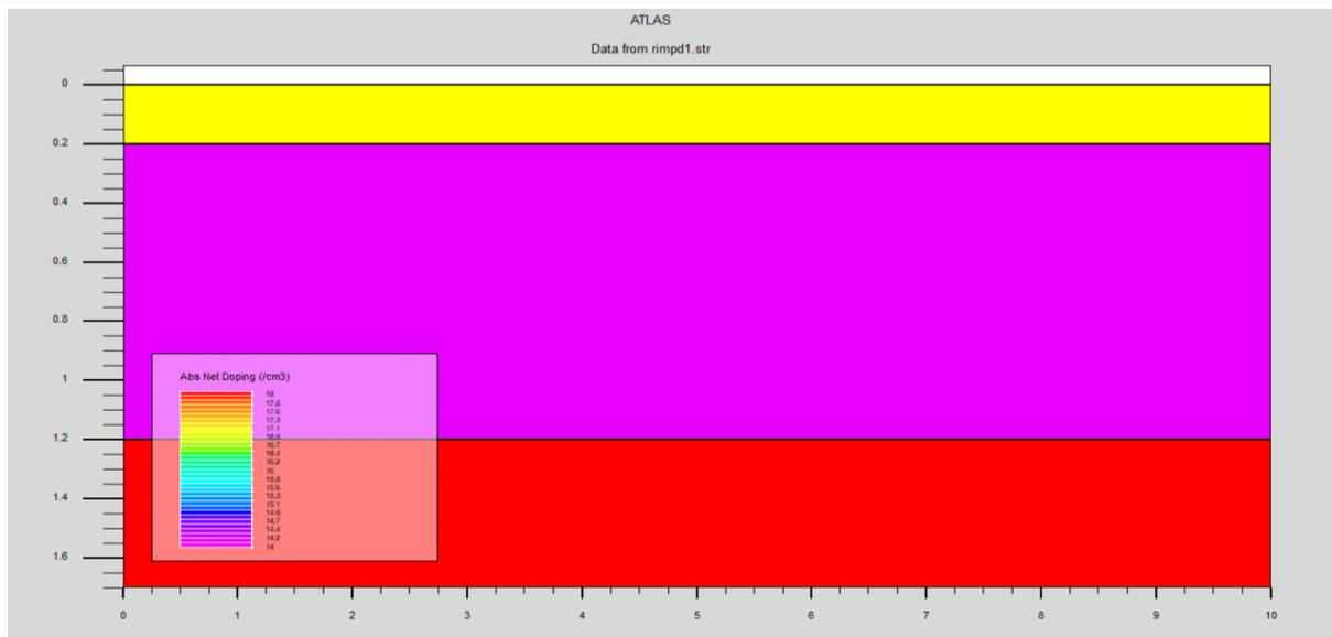
Fig . 3.4 Doping concentration of PIN photodetector
