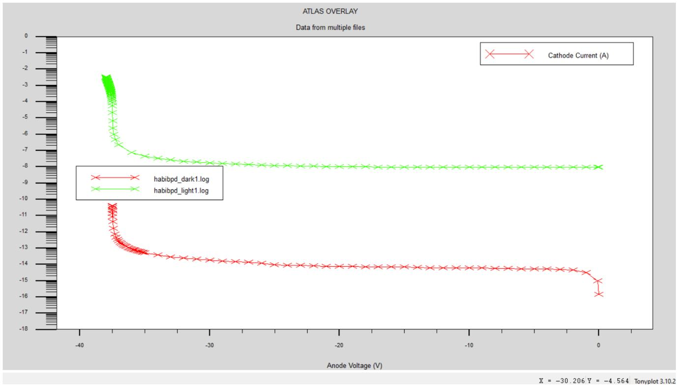
Fig . 5.4 cathode current vs anode voltage under light and dark conditions
