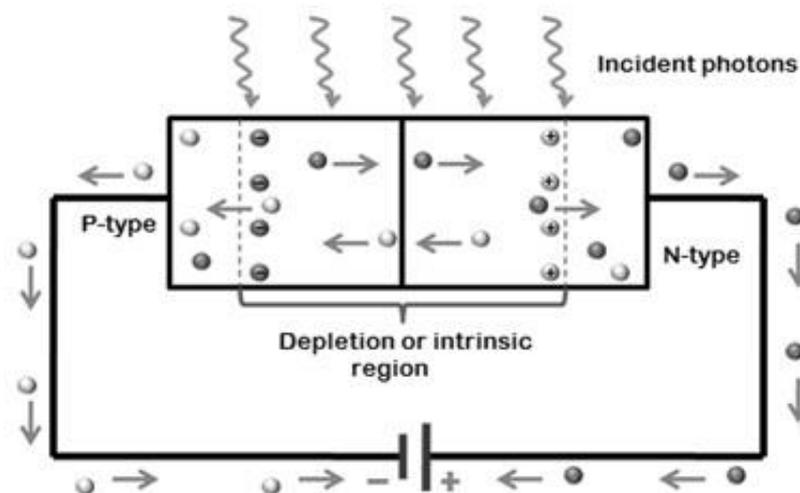
Fig : 2.1 Working Principle of photodetection
