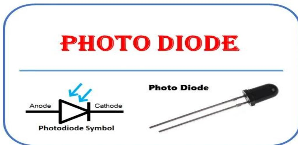
Fig 1.1 photodiode
